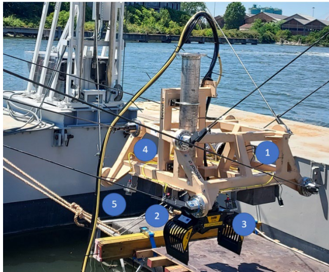
Figure 6 - Location of the 5 IP cameras in the underwater robot frame
