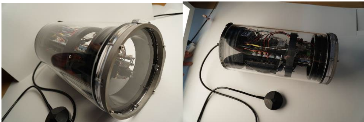
Figure 7 – The waterproof underwater capsule of the smart camera system
